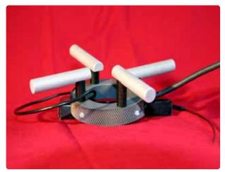
Figure 1. The CorroWatch probe
