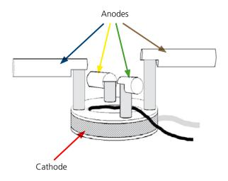
Figure 2. CorroWatch probe structure. The black cable is the reinforcement connection cable.
