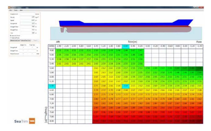
SeaTrim 3 from FORCE Technology makes it possible to determine the optimum trim for a given combination of speed and displacement within seconds.
