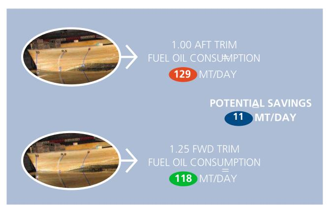
The pictures show a Post Panamax sailing at 20 knots. By sailing with a 1.25 fwd trim, the Fuel Oil Consumption is 8.5 % lower than by sailing with 1.00 aft trim. This equals \$ 6,160 saved per day of operation at a fuel oil price of \$ 560 USD/ton IFO380 (August 2014).
