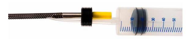
The black interference fit plug has a hole in it through which the grout is injected with a syringe. The clear plastic pipe allows the air to escape and leave a vacuum holding the grout until it cures.
