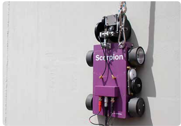
Automated UT-thickness measuring of tank shell – Equipment: Silverwing scorpion crawler
