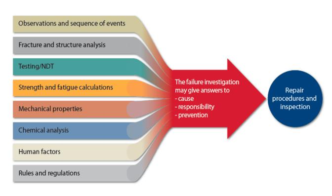
A failure and damage investigation may be dealt with in many ways, depending on the requirements to be met. Sometimes it requires only few and simple examinations to clarify specific technical questions and sometimes a more thorough examination is required, to determine causes etc., called Root Cause Analysis (RCA).
