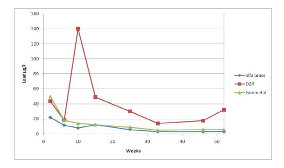
Fig. 3. Lead release after 12 hours stagnation from machined test pieces of alfa brass, dezincification resistant brass (DZR) and gun metal. Average of two data sets.
