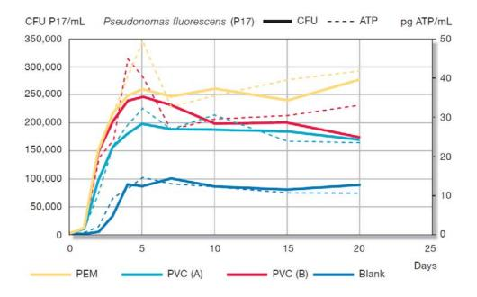
Fig. 7. Growth measured by HPC and ATP of the bacteria strain P17 at 15 °C in drinking water extracts of two types of PVC, a PEM material, and in blank (water alone).[7]
